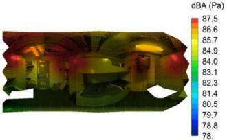
Acoustic array plot BEFORE treatment with Silent Running
